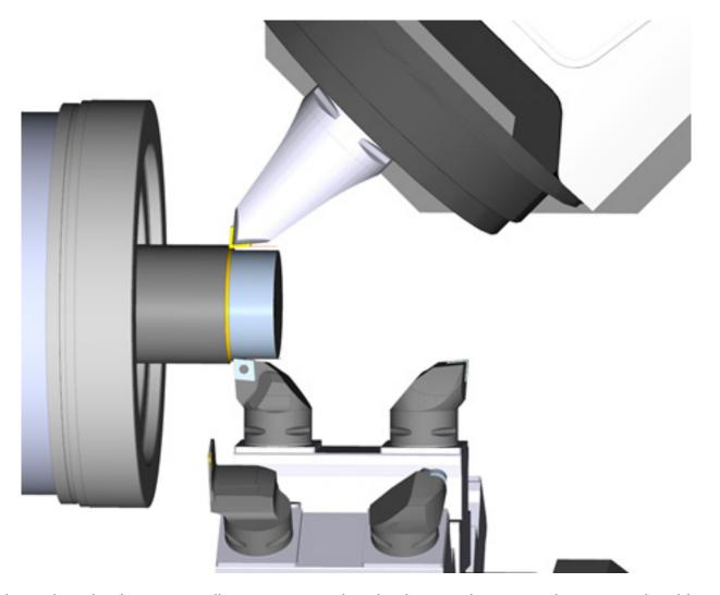
Balanced turning lets you easily program synchronized cuts using two tools on opposite sides of the turning axis. Balanced turning reduces cycle time with simultaneous operations, and reduces part deflection during heavy cuts by supporting the workpiece at both sides. Choose between two balanced turning cycle types:
