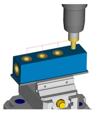
Milling tool control points let you specify a preset or custom control point for each machining cycle. Each milling tool type has one or more predefined control points, and you can specify custom control points along the tool's centerline by distance from the tool tip along the tool axis.
