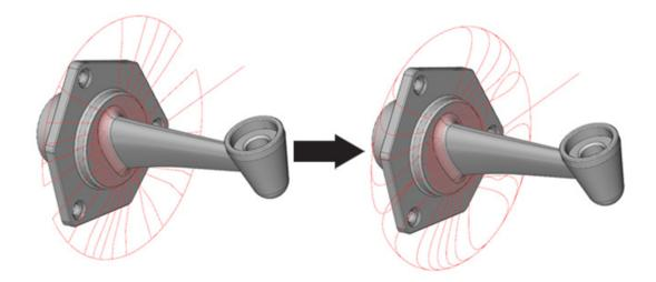
A new rapid link type, Smooth Radial Around Axis, produces continuous smooth motion to:
