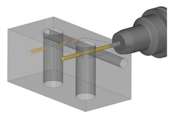
ESPRIT 4.3 supports automatic feedrate adjustments for drilling cycles that encounter existing holes or pockets during the cycle, to minimize burr formation, improve chip evacuation, prevent tool deviation, and reduce tool wear and avoid tool breakage.
