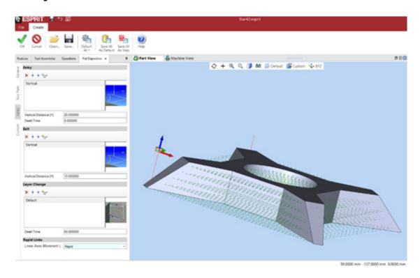
New links settings for Additive cycles provide a dedicated approach/exit for additive trajectories, as well as easy management of dwell times between part layers.
