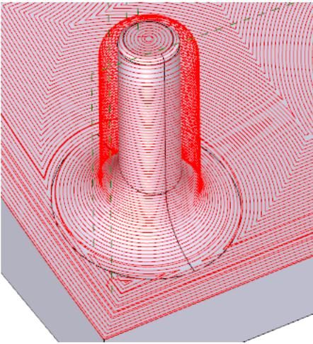
The system first calculates Z-level toolpath on the entire part. All toolpath that flows entirely on areas above the slope threshold is maintained. Toolpath in areas below the slope threshold is replaced with concentric passes. This method gives priority to the continuity of the toolpath, and attempts to preserve uninterrupted Z-level passes as much as possible.
