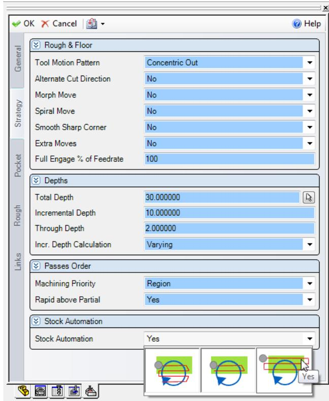
When Stock Automation is set to Yes in the Pocketing cycle, the following parameters will be set automatically by the system and hidden from the user:
