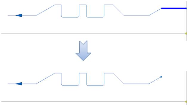
Figure 8. When necessary, previous or next sub-elements are trimmed to the intersection point.
