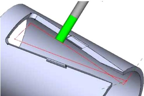
Figure 10. Automatic Curve calculates a curve to keep the tool axis as perpendicular as possible to the feed direction.
