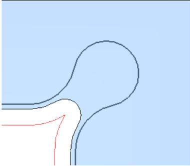
Figure 5. Pocketing on an open profile will rough only the remaining material.
