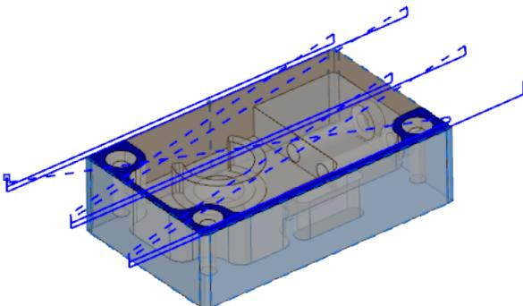
In previous versions, if the stock was a standard block and the shape of the top face was smaller or had a different shape, the user had to take extra steps to create a feature that more closely matched the shape of the stock. The user also had to determine the best distance for the tool to sweep past the edges to ensure a smooth surface all around.
