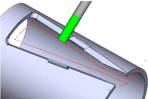
Figure 9. Upper Profile positions the tool to follow the upper profile, automatically shifting the tool along its axis to completely machine the wall.
