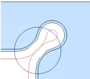
Figure 3. No-core pocketing on the entire profile is inefficient and time consuming.
