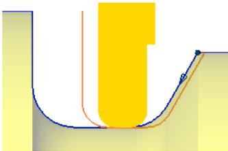
Figure 10. When Control Edge Shift is set to Yes, the control edge is allowed to shift to produce NC code that matches the part drawing. In this illustration, the control edge shifts from right to left.
