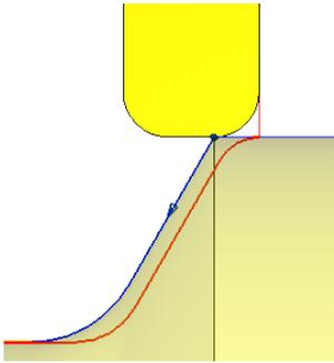
Figure 5. New safety distance for alternating cutting passes.
