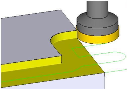
Stock Automation also adjusts the Optimal Cutting Angle if the shape of the stock changes at incremental cutting depths.
