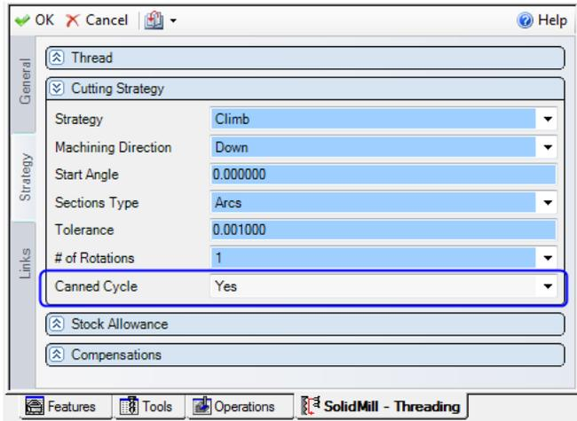
ESPRIT Post Processor has been updated with new examples for support of canned cycle thread milling:
