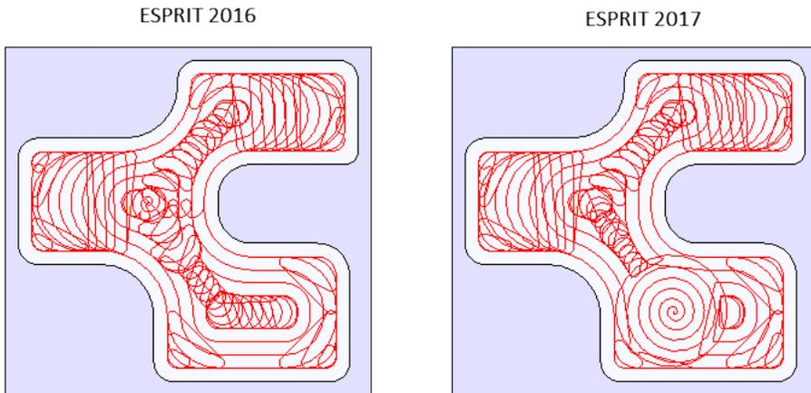
Figure 2. The width of the initial channel is now optimized for the size of the tool for faster cycle times and fewer decelerations.
