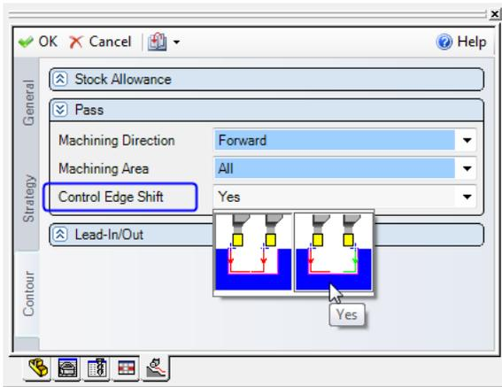
Similar to the Grooving cycle, the Control Edge Shift option has been added to the Contouring cycle. Control Edge Shift can be used to change the position of the tool edge on the tool path from one side to the other in the middle of the pass.
