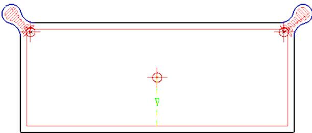
Figure 2. Contouring inside small internal openings can create self-intersecting wire path, possibly violating the profile.
