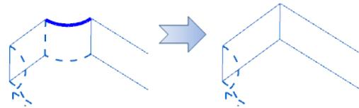
Figure 4. Extended sub-elements retain their original attributes, such as open edges.
