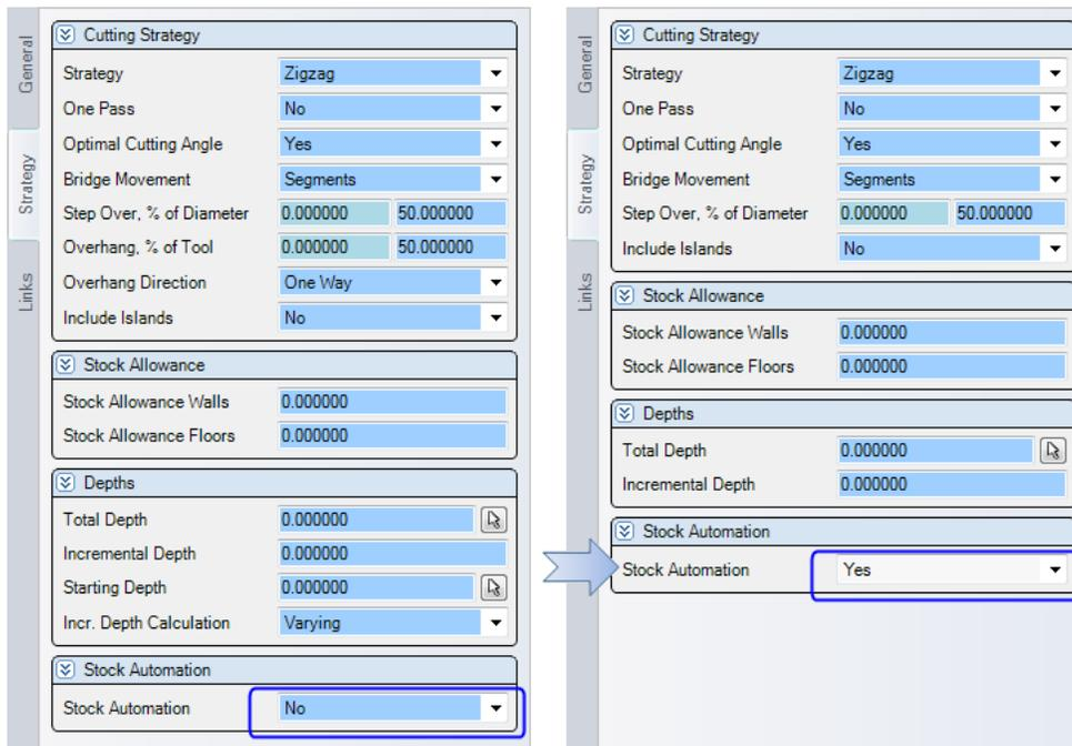
The following parameters will be calculated automatically by the system and hidden from the user.
