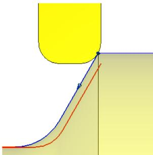
Figure 4. The Blend option adds a blend as the tool enters or exits the feature.
