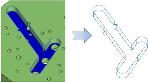
Figure 2. To create smooth walls for a pocketing operation, sub-elements are grouped and deleted to modify the shape of the pocket.
