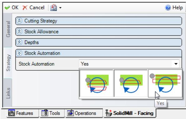
The key to the new optimized facing technology is the completely new Stock Automation engine for milling. Stock Automation now gives the user control over how much automation is applied within the Facing cycle, as well as Pocketing and Contouring:
