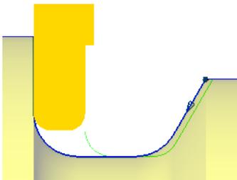
Figure 7. Transition Clearance adds a safety distance to offset the transition point before the tool touches a wall.
