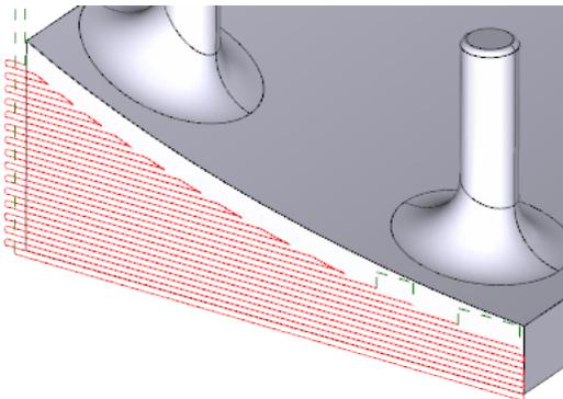
The **Spiral Move** option will apply spiral connections to both Z-level and concentric toolpath. Otherwise, toolpath is connected with an "S" shaped trajectory.
