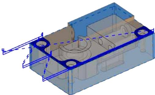
*Figure 2. Now, when a face is selected, the system will calculate the ideal toolpath to efficiently remove stock.*
