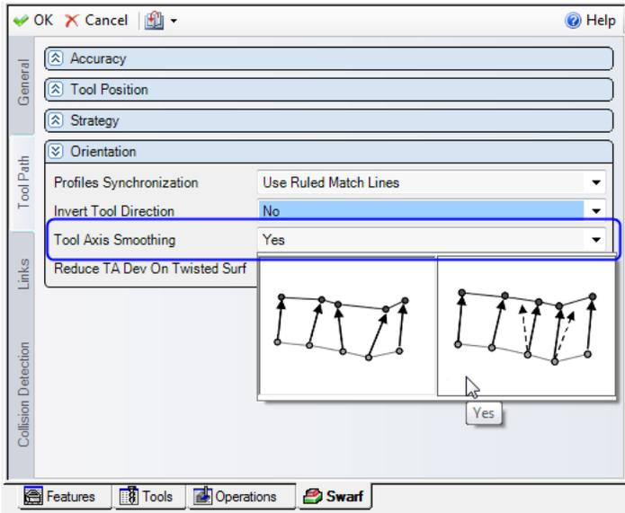
Figure 17. Tool Axis Smoothing acts to smooth the trajectory of the tool axis, reducing the machine axes acceleration and, as a consequence, marks are eliminated.
