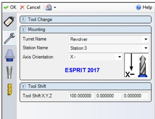
Figure 4. The new option also makes it easier to set up the position of tool stations on the machine.
