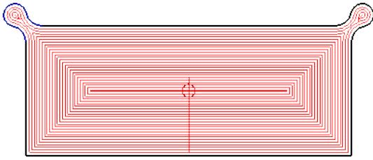
Figure 4. Enabling the Look Ahead function in a contouring operation will avoid small areas where the wire will not fit.
