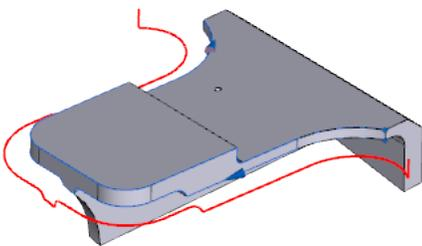
Now the user can control the position of the tool tip to create smooth toolpath even in the presence of irregularities or interruptions of the profiles that define the area to be machined.
