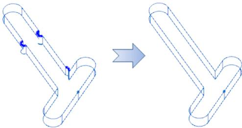
Figure 3. When a sub-element is deleted, previous and next sub-elements are extended and connected to close the gap.
