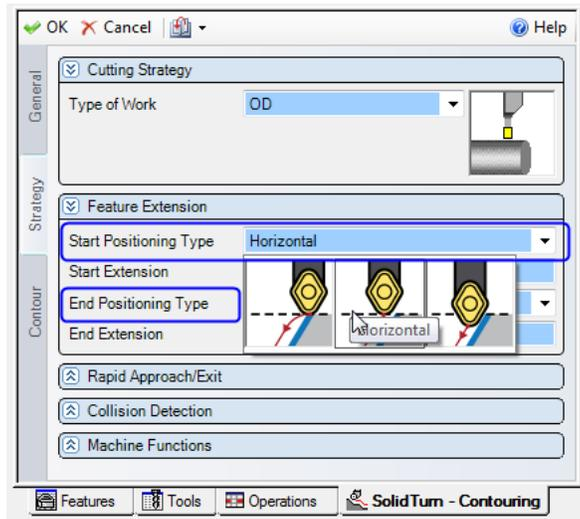
Gain custom control over positioning of the tool at feature start and end points.
