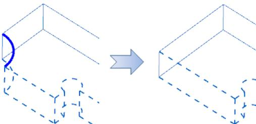
Figure 5. When previous or next elements do not intersect, a new sub-element is created in between. The new sub-element copies the properties of the next element in the feature.
