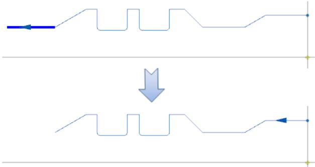
Figure 7. When the starting element is deleted, the feature start point is automatically moved forward.
