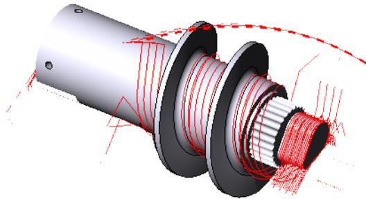
*Figure 3. View entry and exit moves in turning operations.*
