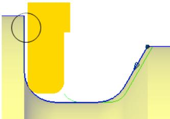
Figure 8. Dynamic change of offset for grooving tools.
