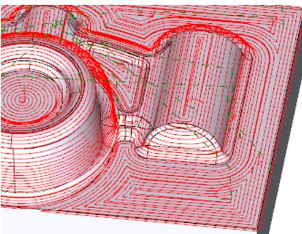
In cases where the part has holes, the option for **Allow Floating Toolpath** will generate toolpath over the openings instead of going around them.
