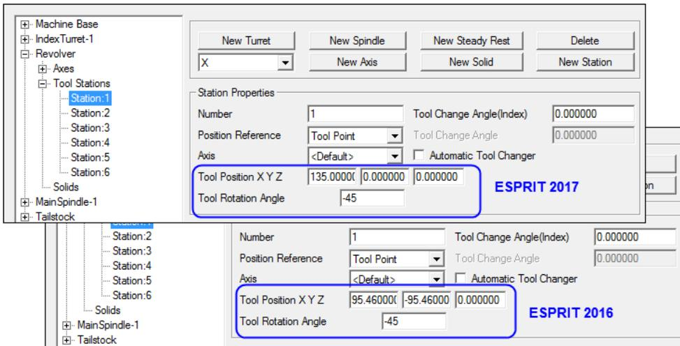
► If you switch Tool Rotation Angle Mode, the system automatically calculates the new tool position on each station. NC code output has been improved to output code without the need for computations inside the post processor.
