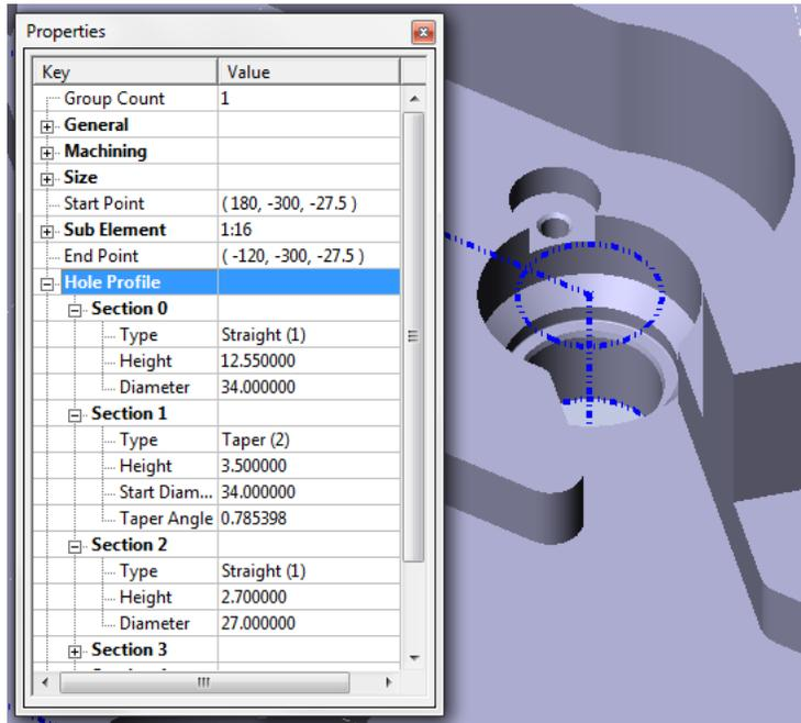
When a hole is too complex to be recognized as a standard hole type (Simple, Countersink, Counterbore), it is categorized as Custom. For example, when a hole has a counterbore as well as a countersink it is recognized as a Custom hole.
