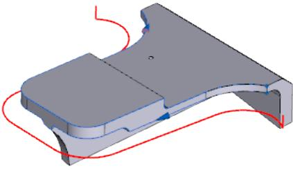
Figure 7. New Tool Reference settings offer a range of options for positioning the tool tip between the upper and lower profiles.
