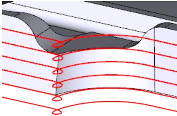
*Figure 2. The new Constant Height Continuous option maintains a constant height even when there are gaps in the part geometry.*
