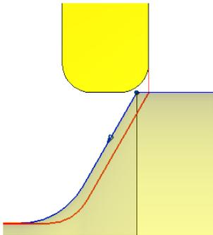
Figure 3. The Normal option places the touch point of the tool at the feature start or end point.
