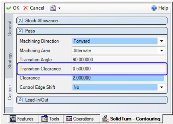
When Machining Area is set to Alternate, contouring passes alternate between vertical and horizontal passes. A transition angle of 90 degrees is used to cut vertical walls. As the tool approaches a vertical wall at the end of a horizontal pass, it can become enveloped in material and risk damage to the tool.
