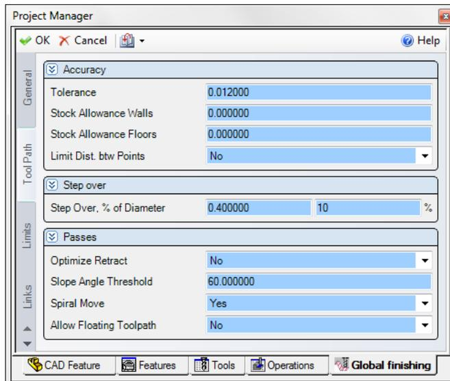
Areas of the part having a slope above the **Slope Angle Threshold** are considered steep; areas below the threshold are considered shallow.
