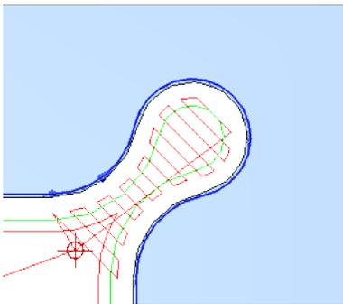
Figure 6. Changing the operation order to perform pocketing between rough and skim cuts results in more efficient wire path.
