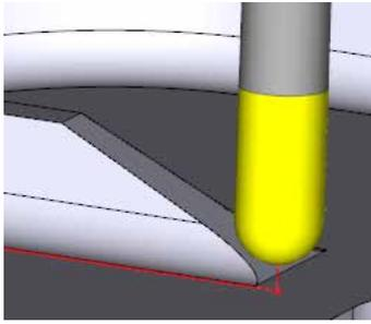
Figure 4. New Tangent Pass Extension settings extend the start or end of the toolpath tangent to the surfaces.
