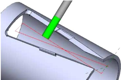
Figure 12. Stop at Floor protects floor surfaces. The tool stops when it reaches the bottom of the wall.
