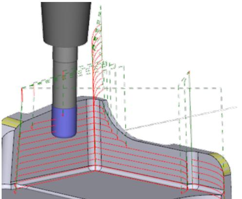
Figure 14. Enhanced toolpath calculation finds tool touch points more accurately.
